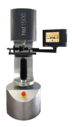
HTD1500 and HTD4000 case hardness depth analyzers deliver quick, accurate, and non-destructive thickness verification up to 1.3 mm (HTD1500) and 2.7 mm (HTD4000)
