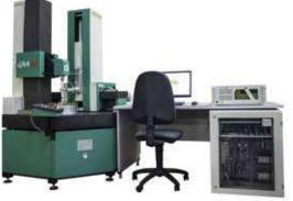
It is a machine with high-level dynamic features thanks to the use of linear motors with pneumostatic supported tracks, which allow movement without any friction. The structure includes three linear axes (X, Y, Z), a rotary axis (W) and a tailstock column, everything based on highaccuracy granite tracks. This permits a better long-term stability and a low thermodynamic response, even in case of temperature variation
