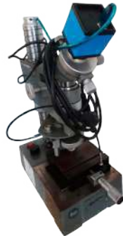
LEITZ (camera – software separated cost) MOD. MINILOAD 1 HV 0.01-0.025-0.05-0.1-0.2-0.3-0.5-1 Test Load: 10-25-50-100-200-300-500-1000 gr
