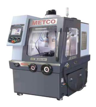
Automatic extra large cutting machine with integral sliding door. Standard Y axis automatic movement, optional Z axis automatic movement. Pulse cutting, step cutting, etc., for burn-free cutting. Preset parameters for consistency and ease of use.
