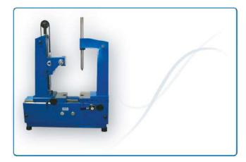
Gears engagement testing is a functional control; we can offer both single-flank and double-flank gear testing machines. The double-flank ones are recommended for the test of spur gears; the single-flank instruments, instead, are recommended for the control of spur gears, bevel gears and worm gears. The test is performed with either a measuring master or a torque gear.
