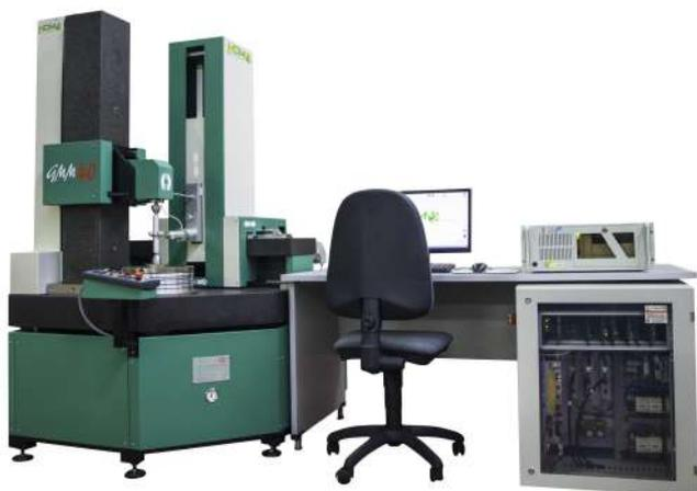
MISURA INGRANAGGI CON DIAMETRO ESTERNO FINO A 400 mm
